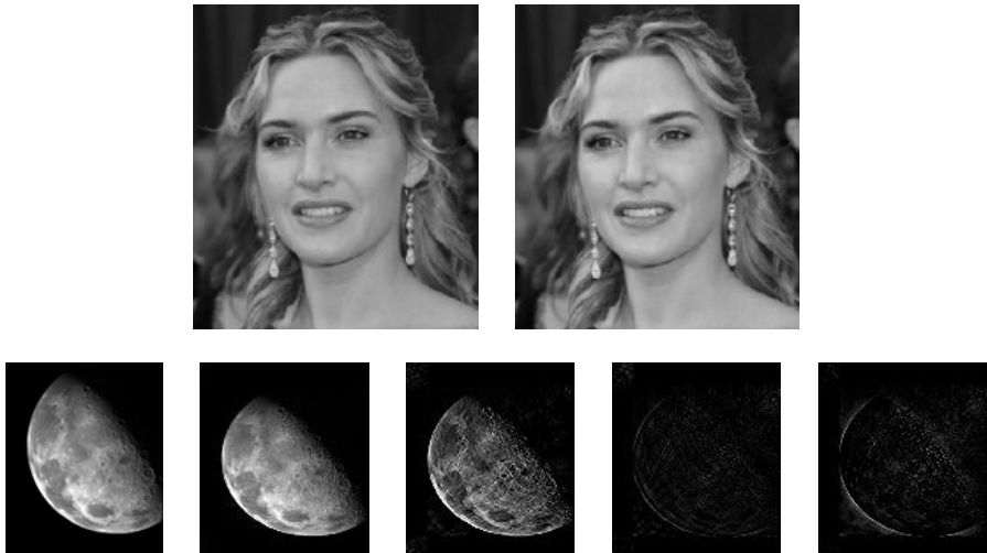
Fig. 5. (a). Top Row from left: Cover image and watermarked image (b). Bottom row from left: Original watermark and extracted watermarks from four quadrants.
