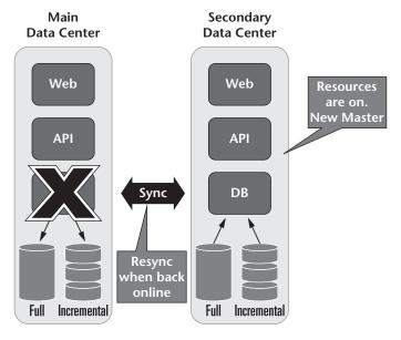
Figure 13.3 Redundant Data Centers—Active-Passive Warm
