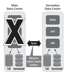
Figure 13.4 Redundant Data Centers—Active-Active Hot
