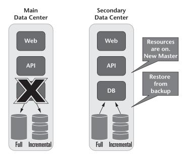
Figure 13.2 Redundant Data Centers—Active-Passive Cold
