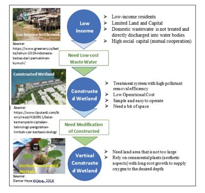
**Figure 2.** Diagram of Possibility Study of Implementing Vertical Constructed Wetland for d domestic wastewater treatments in urban Kampong *Source: Private Documentation*
