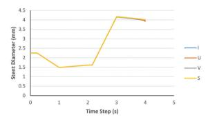
Figure 3. Diameter of stent changed during simulation
