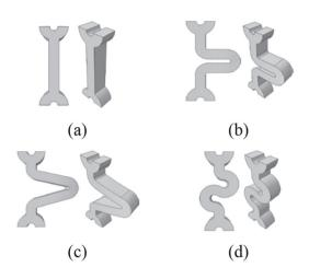
Figure 1 Four stents with different strut linker geometry: (a) I-shaped, (b) U-shaped, (c) V-shaped, and (d) S-shaped
