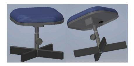
Figure 2. The 3D Model of the Adjustable-Ergonomic Chair
