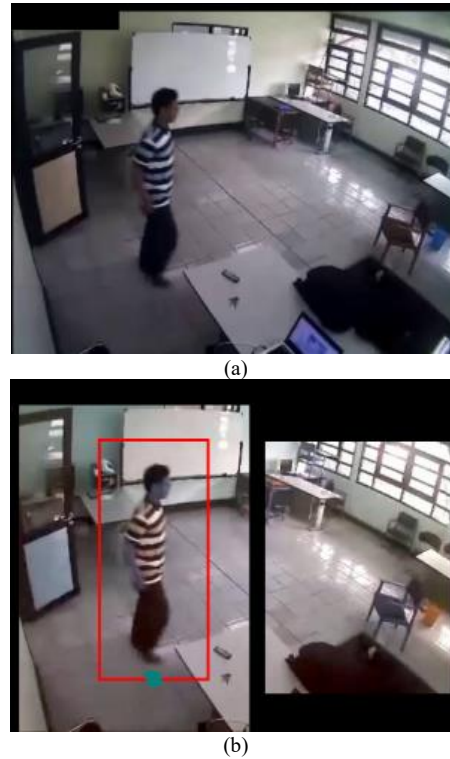
Figure 10. Human Detection in the sample frame using MSR and Linear-SVM: (a) original (b) enhanced using EFF.
